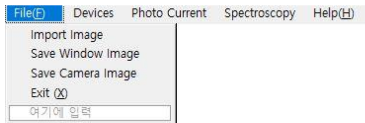
Figure 5 "Save Window Image" or "Save Camera Image" at the File menu to save optical images
